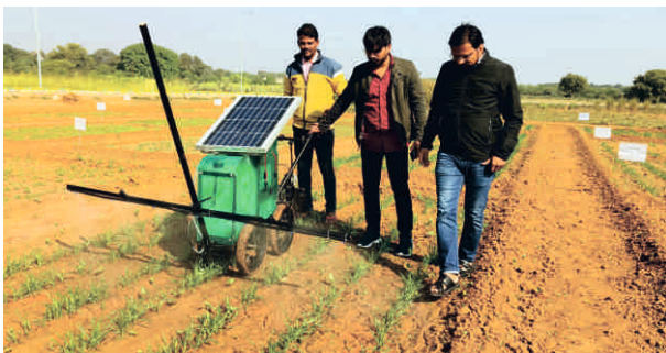
Fig. 3.5.7 Solar-powered self-propelled multipurpose machine developed by institute
