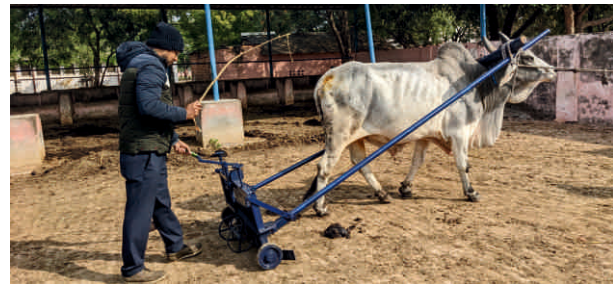
Fig. 3.5.8 Developed animal-drawn shed scraper
